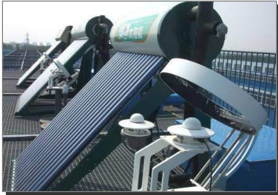
Thermal performance test platform
